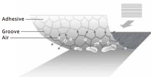
Air trapped between the BELBIEN and the substrate exits through specially designed narrow grooves as pressure is applied with the squeegee.
